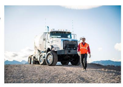
infrastructure projects. Since ready mixed concrete typically only has a 120-minute shelf life from the time of initial batching until it must be completely unloaded from the concrete truck and placed in the formwork on the jobsite, our industry is a local industry that hires local workers to support the local construction economy.
